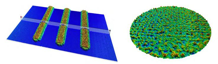
Printed biosensor analyzed using FocalSpec Map software. 3D view of profile extractions for step-height measurement (left) and roughness inspection (right).
